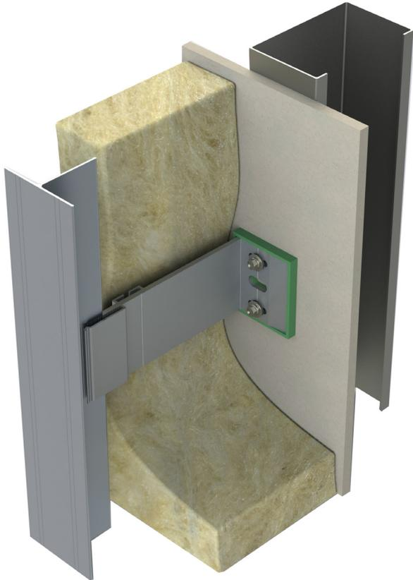
NVELOPE® VB / HB aluminium brackets are supplied with a green plastic “isolator” which offers a degree of thermal benefit. However its principal function is to eliminate any potential of galvanic corrosion between masonry and aluminium substrates.
