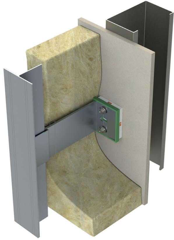
Whilst strong and easy to install aluminium is very thermally conductive e.g  $> 200 \text{ W/mk}$ . Therefore the thermal point loss affects can be significant when aluminium brackets are utilised depending on the combination of various elements within the rainscreen build-up.
