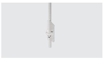
5. Insert toggle with care through baseplate and drilled hole in roof, ensuring the toggle doesn't deploy until it has cleared the deck. Using toggle tubes prevents early deployment within the roof build up.
