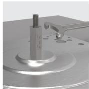
12. Drop baseplate into position over protruding studs.
