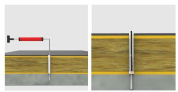
2. Using a 14 mm diameter hole saw or auger bit, drill through the insulation in 4 locations.
