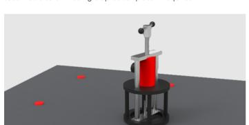
16. Turn Highfix lower body onto female boss in baseplate by hand firstly then to the desired tightness with the 19mm spanner until Highfix is seated correctly.
