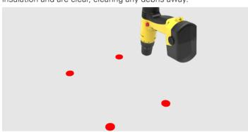
6. Using a wire brush and blow pump remove all debris remaining in each of the four holes.
