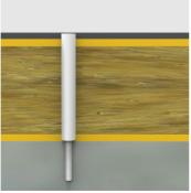
7. Turn studding into screw head of each fixing ensuring the correct stud length is used to allow enough to protrude from the opening to fit a nut and washer.
