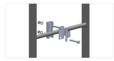
4. Swage/crimp the end toggle to wire and mount bracket.
