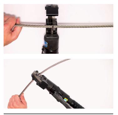
3. As the wire is now cut to the correct length, the tensioner can be removed from the start component ready for crimping/ swaging.
