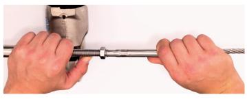
13. Moving down the termination, four more crimps need to be performed, ensuring there is a 1mm gap between each. It is also advised to turn the termination after each crimp so that they are not pressed in the same plane which will prevent the termination from slightly bending.
