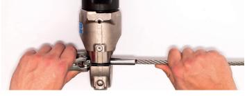
11. Turn the crimper barrel to 'open', pump the handle once to release the jaws.
