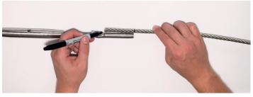
7. Re-insert the wire fully ensuring the wire is fully engaged in the termination up to the point marked.
