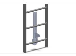
2. Attach with the U clamps provided and torque to 42Nm.
