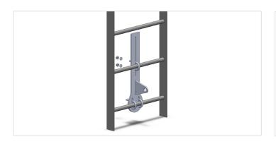
3. Intermediate brackets to be installed at a maximum distance of 6m. (Brackets should be set an unequal spacings to prevent harmonic oscillation.)
