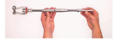
2. Fit the tensioner to the start component loosely, and whilst pulling the wire taught, mark the wire with a marker pen against the pressing on the tensioner. You can now cut the wire on the marking with the Cembre HT-TC026 hydraulic cutter. This will ensure the wire is cut correctly.
