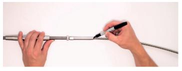
5. Remove the wire and place alongside the termination up to the point just marked.
