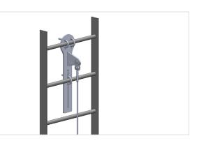
5. Descend the ladder passing the wire through any intermediate bracket.
