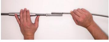
6. Now mark on the termination where the wire ends. This shows where the hollow part of the termination ends, and where the first crimp will be located. This needs to be done on all terminations - tensioners and toggle fork ends.
