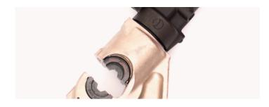
9. Position the central section of the die so that the first crimp is made next to the line marked on the termination itself.
