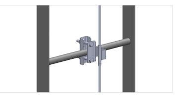
6. Cut, swage and tension wire to appropriate length as detailed on page 8.
