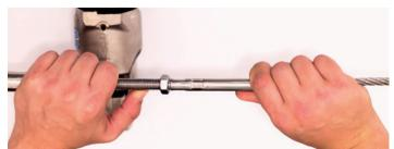
13. Moving down the termination, four more crimps need to be performed, ensuring there is a 1mm gap between each. It is also advised to turn the termination after each crimp so that they are not pressed in the same plane which will prevent the termination from slightly bending.
