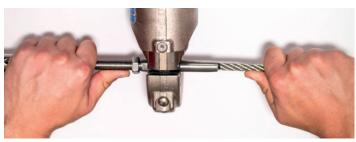
14. All five crimps must be completed on the straight shank hollow section of the termination, and before the chamfered end. Each crimp should show the A10 stamp clearly and not overlap.
