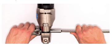
11. Turn the crimper barrel to 'open', pump the handle once to release the jaws.
