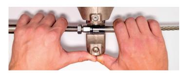
10. During the first crimp ensure that the wire is held into position so that it doesn't slip. Pump the handle on the crimper until a distinctive 'click' is heard and pressure is released from the crimper.
