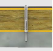
7. Prepare Fischer Vinylester resin tube, nozzle, and gun ready for application. Extrude enough resin through the tube on a test area ensuring the 2 chemical parts are correctly mixed.
