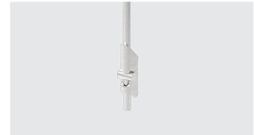
5. Insert toggle with care through base plate and drilled hole in roof, ensuring the toggle doesn't deploy until it has cleared the deck. Using toggle tubes prevents early deployment within the roof build up.
