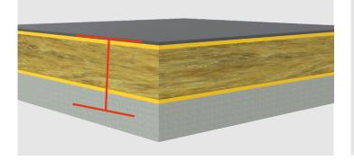
5. Using a SDS Masonry Drill and specified diameter drill bit, drill 4 no. holes into the concrete deck to give the required fixing embedment. If screed is present above concrete deck, remove this first using a larger drill diameter ensuring correct fixing embedment is in concrete substrate ONLY.
