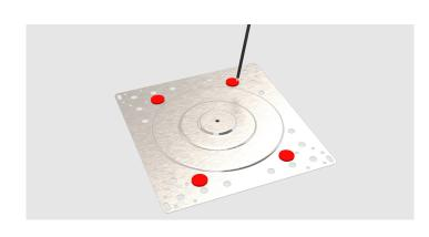
2. Using a hole saw or auger bit, drill through the insulation in all four locations.
