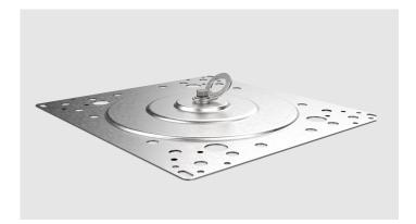
SFS base plates have a central raised dome, complete with a welded M10 female boss, into which the Anchor Point is securely attached. This weld is completely weather tight. Base plates to be used on metal roofing applications come complete with pads on the underside to seal the base plate to the roof sheet crown.
