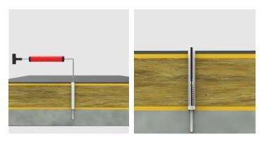
6. Using socket and extended drive bar fasten each of the screws into the concrete deck.
