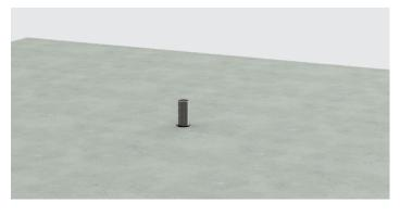
6. Allow for resin to cure based on temperature/conditions on site. See tube for indicative curing and setting times.
