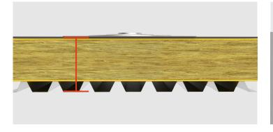
2. Push screws fully into Sleeves, through the plate and into the insulation.
