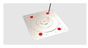
2. Using a 14 mm diameter hole saw or auger bit, drill through the insulation in 4 locations.
