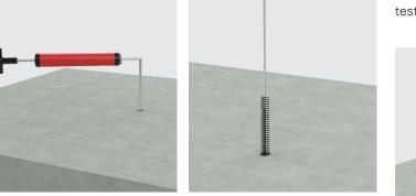
3. Prepare Fischer Vinylester resin tube, nozzle, and gun ready for application. Extrude enough resin through the tube on a test area ensuring the 2 chemical parts are correctly mixed.
