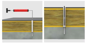
7. Prepare Fischer Vinylester resin tube, nozzle, and gun ready for application. Extrude enough resin through the tube on a test area ensuring the 2 chemical parts are correctly mixed.
