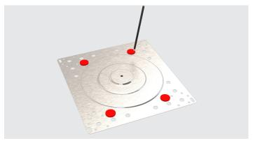
2. Using a 25 mm diameter hole saw suitable for the deck construction, drill through the insulation and deck in all four locations. Ensure all four fixing holes have been drilled through the total roof build up and are clear, clearing any debris away.
