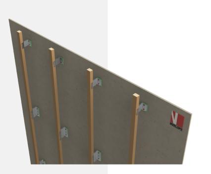
NVELOPE brackets are secured directly to a new or existing substrate of; concrete, brickwork or blockwork or steel frames. Suitable primary anchors are employed to position the brackets to a pre-determined grid to suit the panel layout – please liaise directly with preferred NVELOPE Primary Fixing supplier re pull-out.
