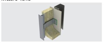
NVELOPE® VB/HB aluminium brackets are supplied with a green plastic "isolator" which offers a degree of thermal benefit. However, it's principle function is to eliminate any potential of galvanic corrosion between masonry and aluminium substrates.
