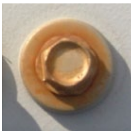
Corrosion of nitrided stainless
