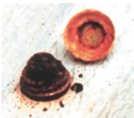
Push fit cap accelerating corrosion
