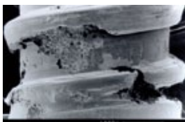
Stress cracks in modified martensitic stainless
