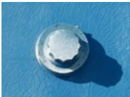
UV fading of moulded heads
