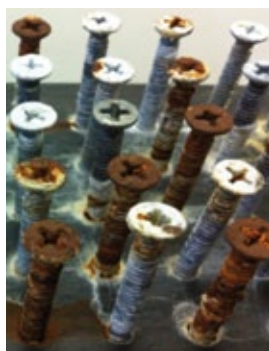
Corrosion of coated carbon steel under Kesternich testing
