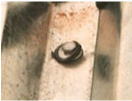
Loose sealing element not retained under head
