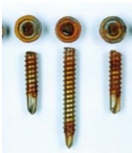
Brittle failure of modified martensitic stainless
