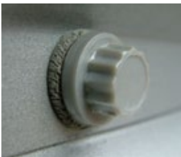
Poor quality EPDM showing UV degradation
